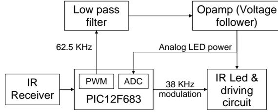
Figure 3: Block diagram of an individual sensor.
