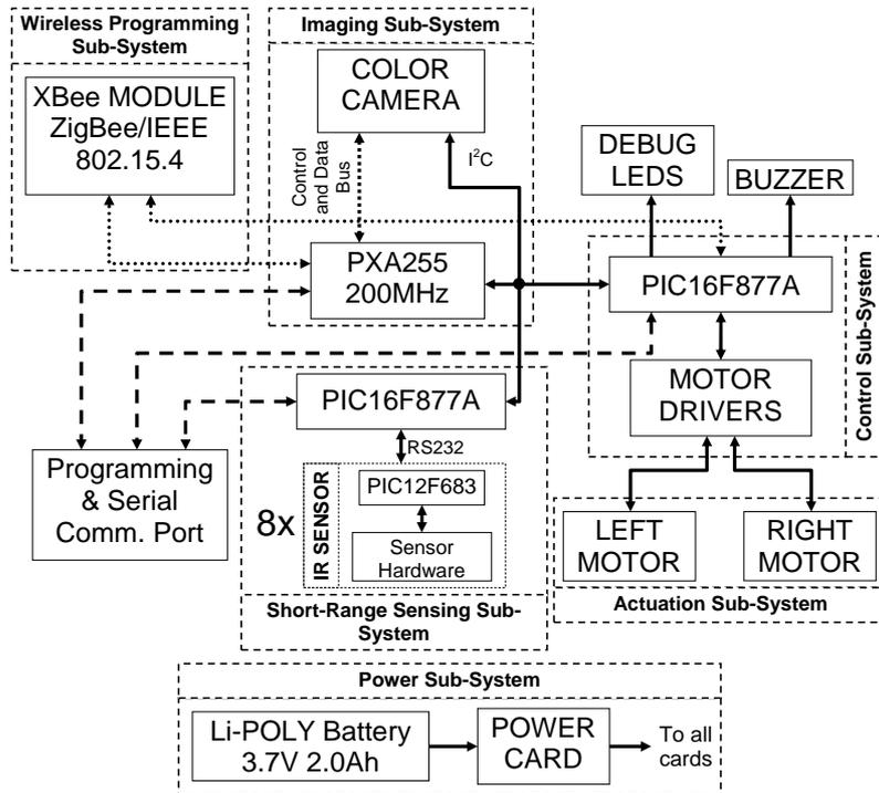
Figure 2: Schematic diagram of Kobot’s control system.
