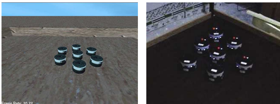
Figure 6: (a)A snapshot from the flocking behavior of Kobots on the simulator (b)A scene showing the real robots performing the flocking behavior
