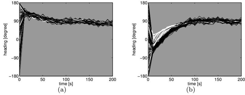
**Fig. 2** Time evolution of the headings of 100 robots in two sample experiments. 10 robots are commanded to go in  $90^\circ$  direction. The traces of informed robots are indicated with white bold lines. (a)  $\gamma = 0.5$  (b)  $\gamma = 1$
