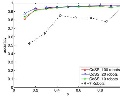
**Fig. 3** Plot of accuracy of flock direction as function of ratio of informed robots for different flock sizes. The error bars are not shown since accuracy is a function of angular deviation.
